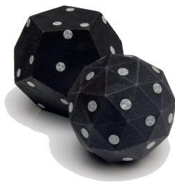
Figure 6.3: Examples of two general-purpose tracking targets. Notice how multiple markers are clearly visible from a single viewing angle.
