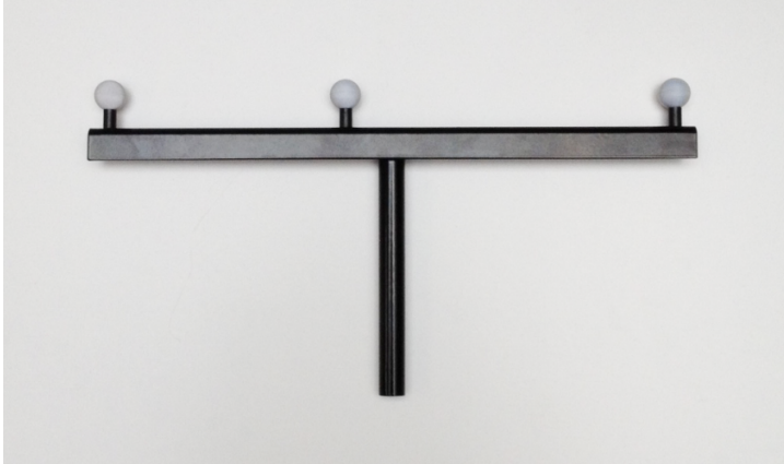
Figure 7.16: Registration device used for setting up multiple PST units
