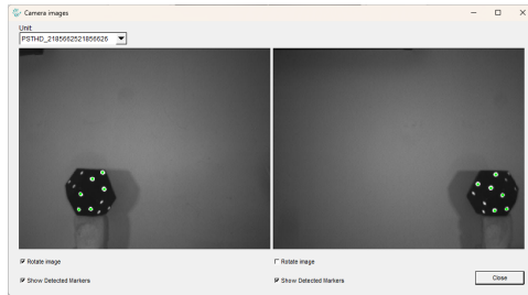
Figure 1.4: Tracker camera view showing optimal target image.
