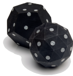
Figure 1.3: Examples of two general-purpose tracking targets. Notice how multiple markers are clearly visible from a single viewing angle.
